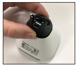
1. Attach the holder connector part to the device socket, following the blue dots.
